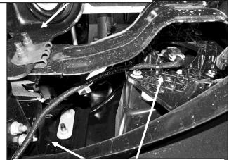
(Fig 2) Release clips attaching the wire harness for fog lights if equipped. Passenger side pictured from behind bumper
