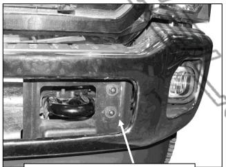
(Fig 3) Remove factory bumper bolts
