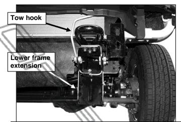
(Fig 4) Remove tow hook and lower frame extension
