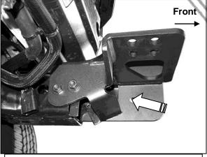
(Fig 8) Insert Bolt Plates into open end of frame (driver/left frame Bracket pictured)
