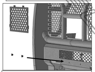
(Fig 24) Remove center screen if equipped with grille mounted camera. Push plastic plugs into holes in Bumper for license plate
