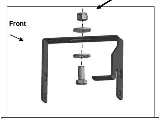
(Fig 16) Rectangular fog light installation (light not included). Attach driver/left Upper Bracket to the slot in top of the opening
