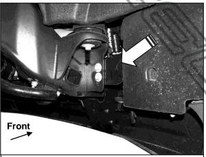
(Fig 3) Remove outer bumper support brackets between frame and bumper (arrow)
