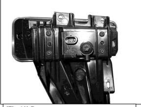
(Fig 19) Remove screws to remove narrow LED fog light from plastic mount
