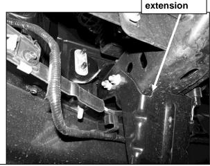
(Fig 2) Release clips attaching the wire harness for fog lights if equipped (driver side)
