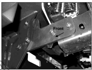
(Fig 23) Attach Bumper to side of Bracket (driver/left side pictured from behind bumper)
