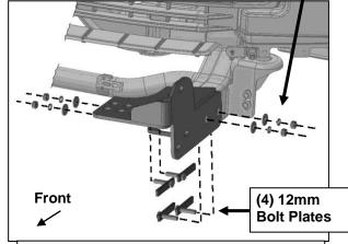
(Fig 7) Insert Bolt Plates into open end of frame. Attach Bracket to sides of frame
