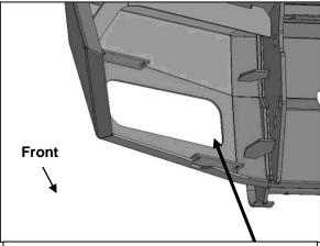
(Fig 20) Remove fog light mount from back of Bumper (driver/left side illustrated)
