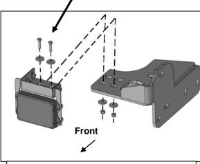
(Fig 15) ACC assembly attached to the Driver/left side Frame Bracket illustrated
