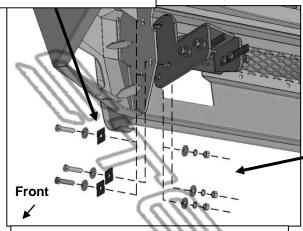
(Fig 22) Attach Bumper to side of Bracket. NOTE: Insert Plastic Washers between Flat Washer and mounting plate on Bumper to minimize corrosion
