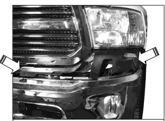
(Fig 4) Remove fascia body panel from top of bumper, (arrows) or 1pc plastic bumper cover
