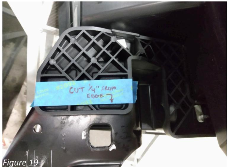
23.\* Using a small reciprocating saw, trim the lower louver shroud as shown. (Figure 20-22)
