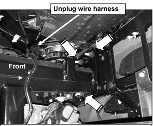
(Fig 2) Remove flange nuts attaching the bumper assembly to the end of the frame (driver/left side pictured from behind bumper)
