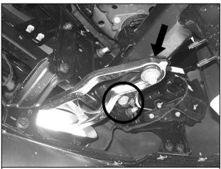
(Fig 4) Loosen but do not remove body bolt (arrow) and remove hex bolt (circle) to remove two hooks (passenger/right side pictured)
