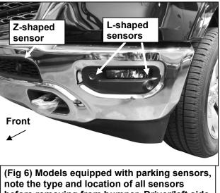
note the type and location of all sensors before removing from bumper. Driver/left side sensor location pictured with factory bumper on for instruction purposes only
