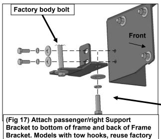
hex bolt to attach Bracket to bottom of frame
