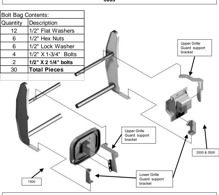
**Step 1:** Raise the Hood. Remove the two nuts on the side of the frame behind the frame cap (2500, 3500). Remove the two or three nuts on the back of the frame cap (1500). Insert upper grille guard support bracket and align to the two bolts, replace nuts and tighten. (Hint: the bracket should be below the hood 3/8" when the hood is closed).
