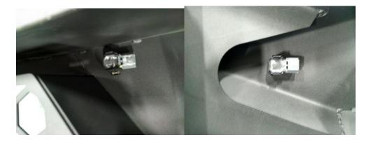
F. Prep the area shown below and attach the red LED strip in the location shown. Wire as desired depending on functionality. You have the following options: wire to your brake lights, running lights or tag lights.
