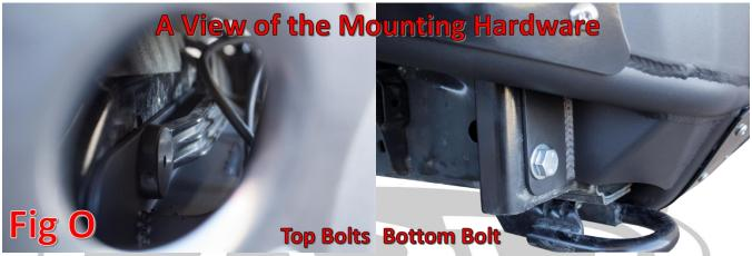
5. Line the bottom mounting holes on the skid plate portion of the front bumper up with the U-nuts you installed in Installation Step 3. Loosely install the supplied 3/8" Hex Head Bolts (x2) and 3/8" Washers (x2). (Fig P)
