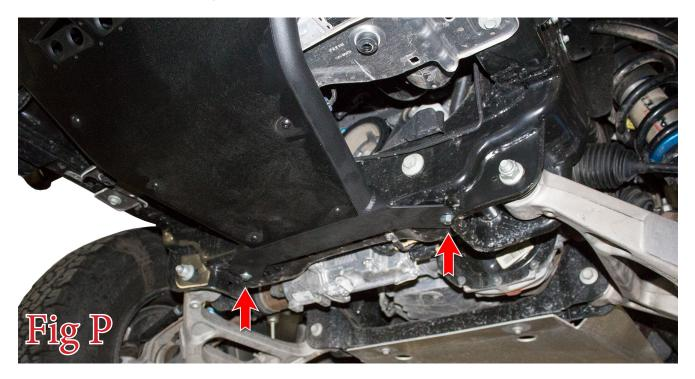
18. Align your bumper so it is centered left to right and sits straight in relation to the vehicle's grille/valance. Then, tighten the 1/2" mounting bolts to 70 foot pounds and the 3/8" mounting bolts to 25 foot pounds.
