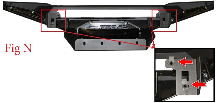
19. Choose the appropriate skid plate mounting bracket for your vehicle. If your vehicle has a lift kit, you will use a different bracket than if your vehicle has stock suspension. Refer to (Fig O) to see which one to use.
