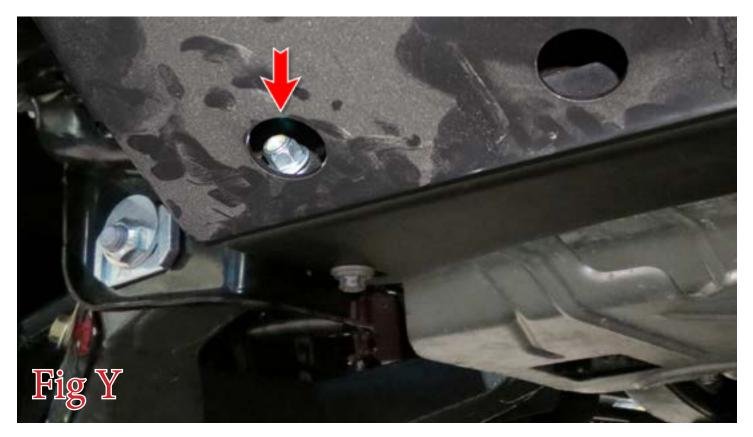
30. Align your bumper so that it is centered left to right and straight in relation to the vehicle's grille/valance. Then, tighten the 3/8" mounting bolts to 25 foot pounds. Tighten the upper 1/2" mounting bolts to 70 foot pounds. Then, lift up on the lower portion of the skid plate until the side wings of the bumper are straight in relation to the vehicle's body. Then, tighten the 1/2" lower skid plate bolts (from Step 29) to 70 foot pounds.
