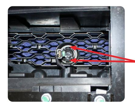
Spread these two tabs to release the parking sensor from its mounting
