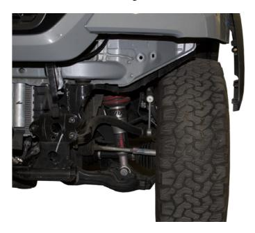
22. Use a utility knife (or something similar) to trim the two black plastic pieces just above the vehicle's frame horns as shown in (Fig V).
