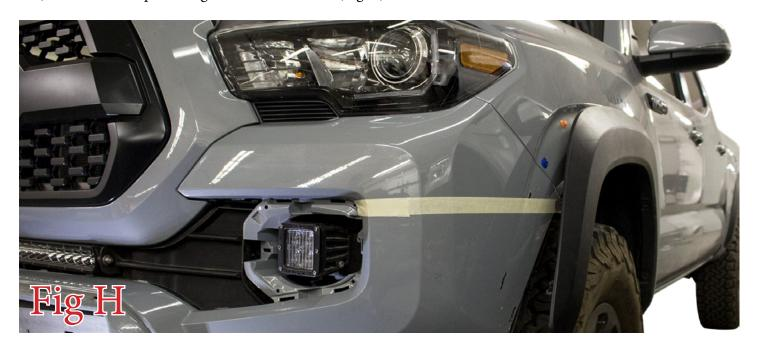
10. When you cut this line, leave about 1/4" of material to ensure you do not cut off too much material. (Fig I)
