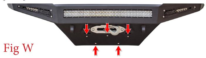
26. Start the first two winch bolts all the way down in the slots until they are finger tight. Then, slide the winch up and start the remaining two bolts. (Fig X) For wiring/operation information, refer to the winch manufacturer's installation guide. Once the winch is installed, reinstall your skid plate.
