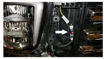
4. Remove the factory side brackets. There will be (3) 15mm bolts per each side.
