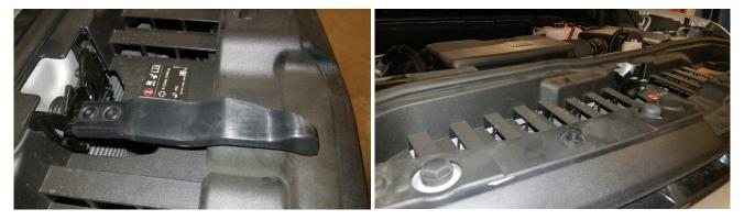
3. If vehicle is installed with a front camera, unhook the pigtail connector. The grille can then be removed by removing the (4) 10mm bolts on top and (4) 10mm (two on each side) from each side.
