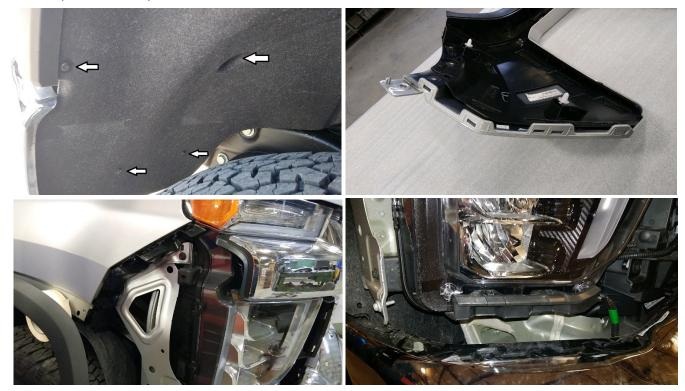
2. Remove the factory grille. Open the hood and remove the hood release latch by removing two T15 screws. Remove the ten plastic clips holding the plastic shield located above the grille.
