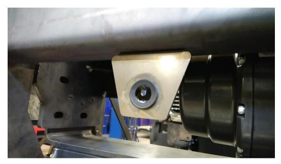
14. Plug in fog light / sensor plug. If the sensor wires are tight, switch the straight outside sensor and the 90-degree sensor (by the fog light) to gain a couple inches.
