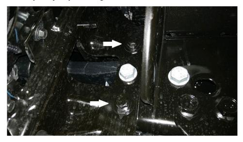
4. Remove the plastic shield that is around the radiator. There will be four 10mm screws and 4 plastic clips.
