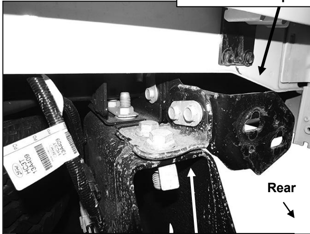
(Fig 4) Remove factory bumper brackets, Do not remove 90-degree support bracket
