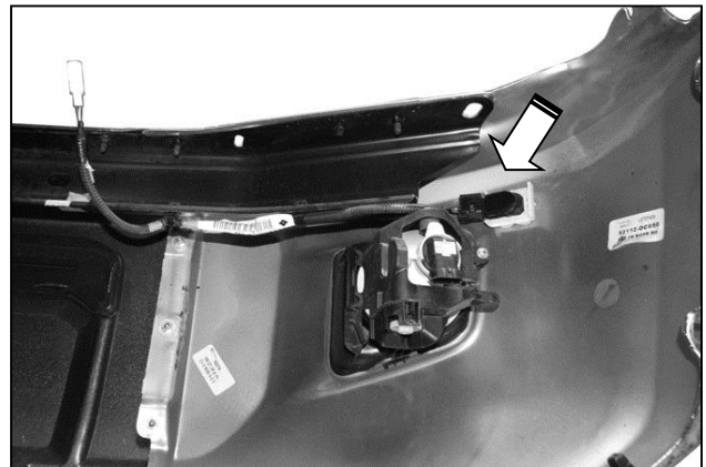
(Fig 18) Slide white plastic cover off sensor. Unplug wire harness. Remove Sensor.
