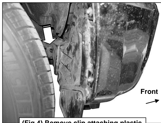
(Fig 4) Remove clip attaching plastic cover to side of frame (arrow)
