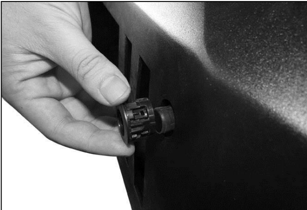
(Fig 19) Push sensor through sensor sleeve on the back of the bumper and attach OE retaining ring to sensor from the front of the bumper
