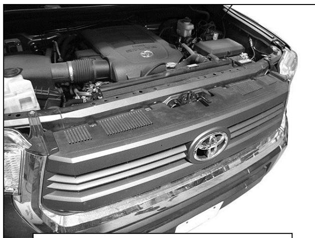
(Fig 1) Remove plastic cover and grille
