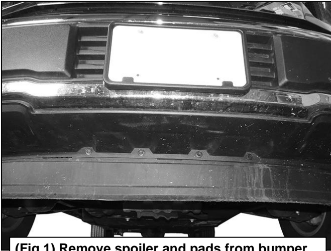
(Fig 1) Remove spoiler and pads from bumper
