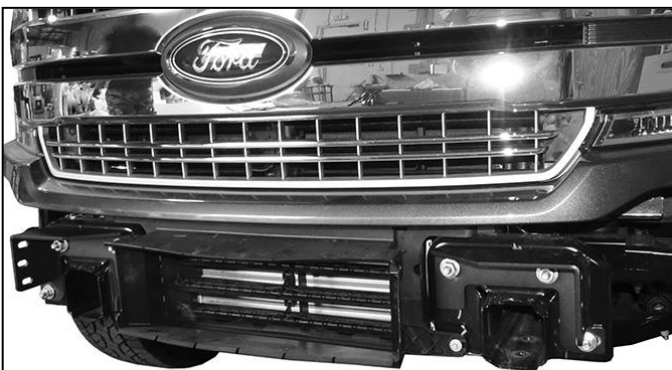
(Fig 4) Attach driver/left Mounting Bracket to end of frame
