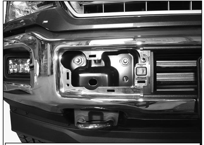
(Fig 2) Remove license plate and plastic bumper pads from bumper (passenger/right side pictured)
