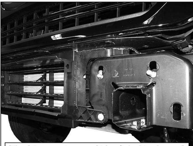
(Fig 3) Remove bumper (driver/left side pictured)
