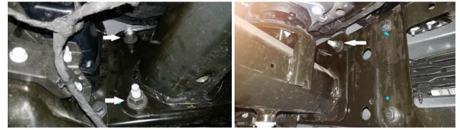
5. Remove the tow hooks (if applied). Loosen the 18mm bolt that goes through the frame to the body mount. On tow hook models, cut off the rubber boot from around the bolt.
