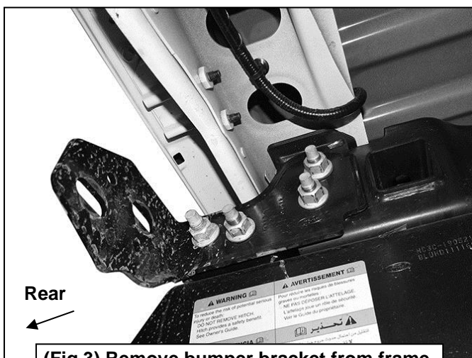
(Fig 3) Remove bumper bracket from frame
