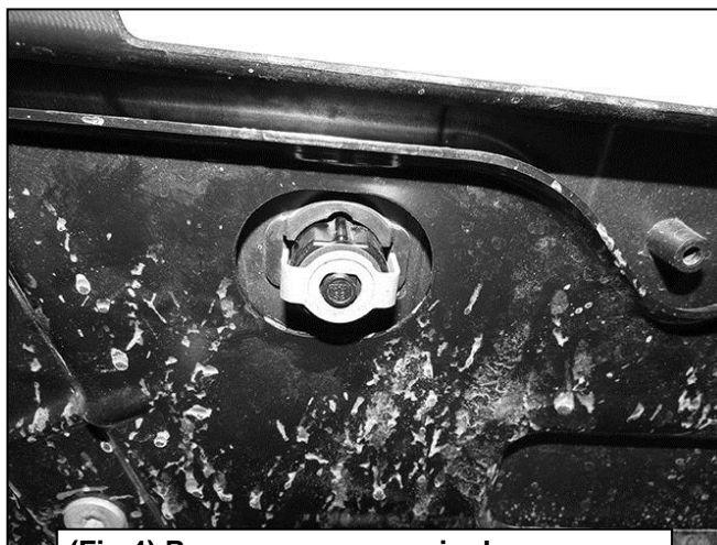
(Fig 4) Remove sensors, wire harness, license plate lights, trailer plug and spare tire access lock (pictured) if equipped
