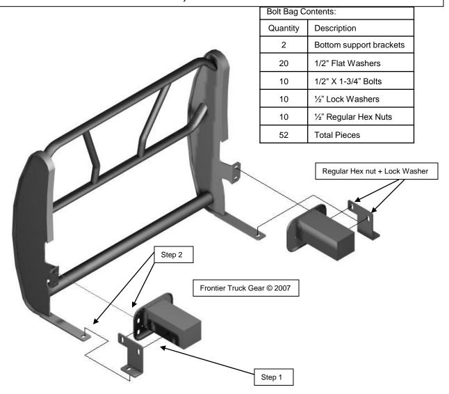
**Step 1:** Install bottom support bracket behind frame horn. NOTE: You must use regular ½" hex nuts and ½" lock washers on the bolts going through the truck frame!! You will access the bolt head through a small hole located on the inside/bottom of truck frame when you are tightening.
