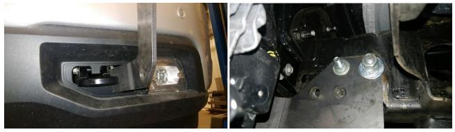
7. Reinstall the tow hooks. Use the factory tow hooks. If there are no tow hooks present, use  $\frac{1}{2}$ " bolts. Also, at this time tighten the 18mm bolt that was loosened in step 1.
