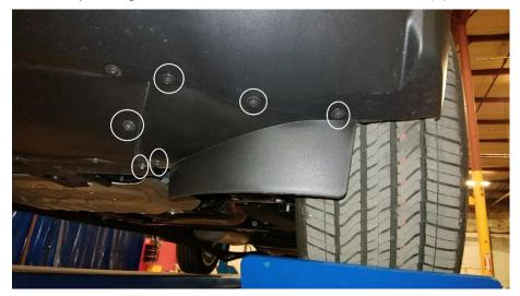
2. Remove the Front Bumper Fascia Deflector. There will be (6) screws on the bottom side and (8) screws on the upper side.
