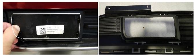
5. There is a driver and passenger side mounting bracket. Mount the brackets to the outer side of the frames. Use 7/16" hardware for the front hole and 3/8" bolt tab and hardware for the back hole. (*Photo shown without lock washers*)
