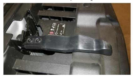
18. Remove the ten plastic clips holding the Air Inlet Grille Panel.
