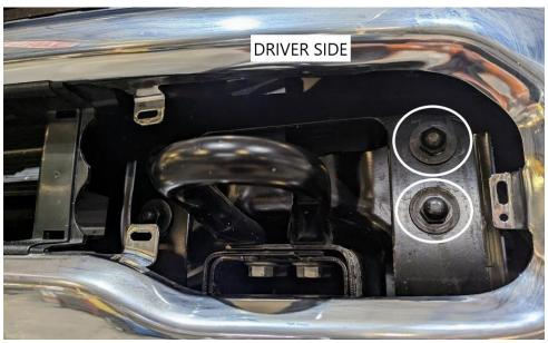
4. To install the bottom bracket, remove the two 18mm nuts from the side of the frame. Install the bottom mounting brackets. Line the top hole of the bracket over the top hole of the bumper. Reuse factory hardware.
