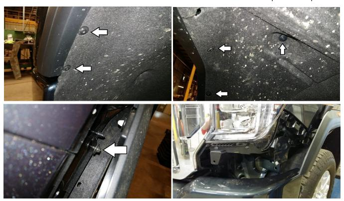
Remove the factory grille. Open the hood and remove the hood release latch by removing two T15 screws.Remove the nine plastic clips holding the plastic shield located above the grille.
