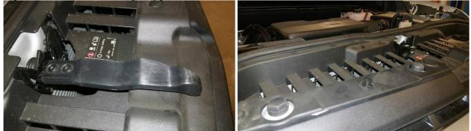
6. If vehicle is installed with a front camera, unhook the connector. The grille can then be removed by remove four 10mm bolts on top.
