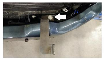
8. Mount the grill guard to the bottom brackets using the black carriage bolts. Set the grill guard to your liking then tighten bolts. Then mount top brackets to the upright of the grill guard and tighten carriage bolts plus the 18mm factory bolt.
