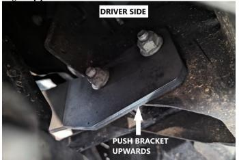
15. To install the top brackets, remove the top bumper bolts. Install one at a time so bumper does not shift. You can access the top bolts either through the lower opening in the grille with a ratchet and 18mm socket with an extension or between the bumper and grille with a 18mm wrench or ratchet wrench.
