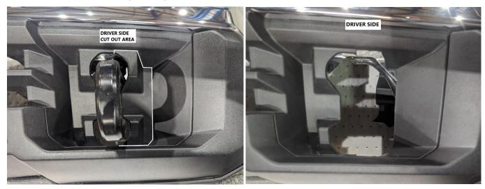
14. Mount the bottom bracket to the outside of the frame. Use  $\frac{1}{2}$ " x 5" bolts to install. Push the bracket upwards and tighten bolts and nuts.
