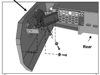
(Fig 18) Attach sensor to Brackets on Bumper
