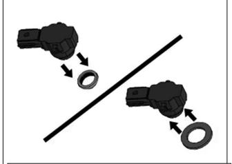
(Fig 11) Models with parking sensors, remove the silicone seal from sensor. Slide Foam Seal over end of sensor (arrow)
