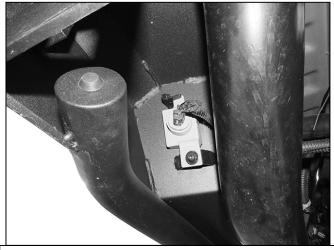
(Fig 20) Passenger/right license plate light installed
