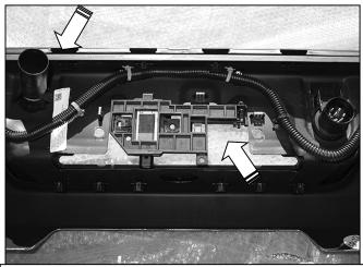
(Fig 8) Remove the sensors, remote antenna with TPMS assembly & spare tire access tube from the back of the bumper. Also remove wire harness.
