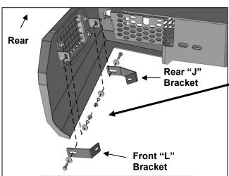
(Fig 17) Attach CTA Brackets to tabs on inside of Bumper
