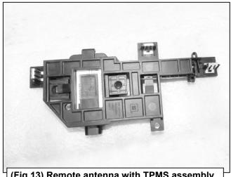
(Fig 13) Remote antenna with TPMS assembly
