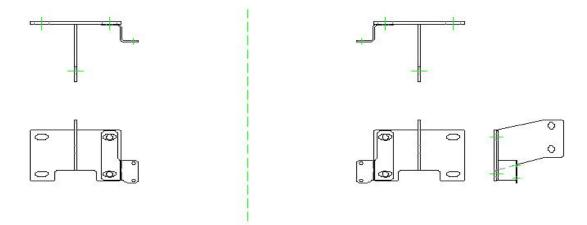
Fasten Ali Arc bumper to Ali Arc steel mounts using supplied bolt kits (4 - 50mm X 12mm) Ensure Ali Arc bumper is sitting level and evenly spaced before completely tightening bolts. Cleaning and Maintenance
