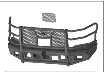
(Fig 20) Remove center screen if equipped with grille mounted camera
