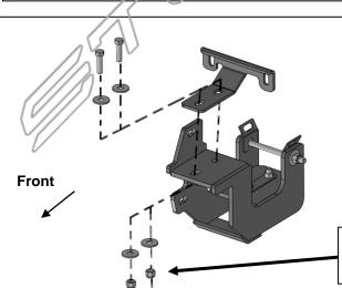
(Fig 9) Passenger side Support Bracket attached to the Frame Mounting Bracket illustrated
