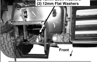
(Fig 8) Attach the Passenger side Frame Mounting Bracket to the Double Bolt Plate
