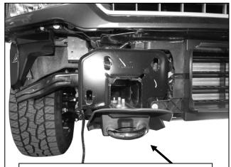
(Fig 4) Remove the passenger side tow hook and plastic cover, (if equipped)
