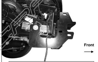
(Fig 6) Insert Spacers between tabs on the Frame Bracket and sides of frame
