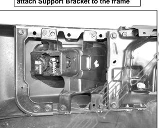
(Fig 12) Remove fog light assembly from bumper
