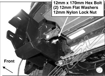
(Fig 7) Slide the Passenger side Frame Mounting Bracket over the end of the frame
