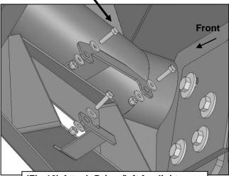
(Fig 16) Attach Driver/left fog light assembly to mounting tabs on Bumper
