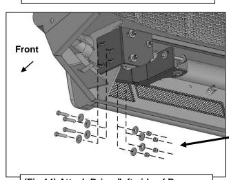
(Fig 14) Attach Driver/left side of Bumper assembly to Bracket assembly (Figure 10)
