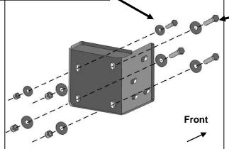
(Fig 7) Attach driver/left Bracket to end of frame
