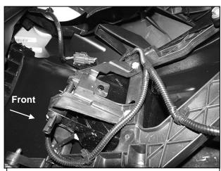
(Fig 4) Unplug lights and sensors if equipped. Unplug harness to bumper and move harness
