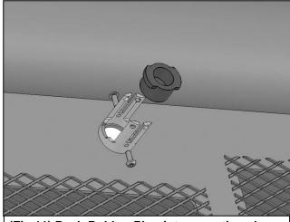
(Fig 11) Push Rubber Plug into mounting sleeve
