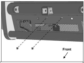
(Fig 18) Attach License Plate Plugs to Bumper
