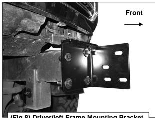
(Fig 8) Driver/left Frame Mounting Bracket
