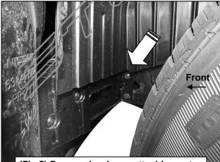
(Fig 5) Remove hardware attaching outer bumper support to side of frame (arrow)
