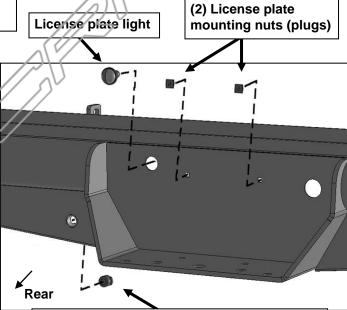
(Fig 8) On models with rear bumper sensors, remove rubber plugs from sensor holes
