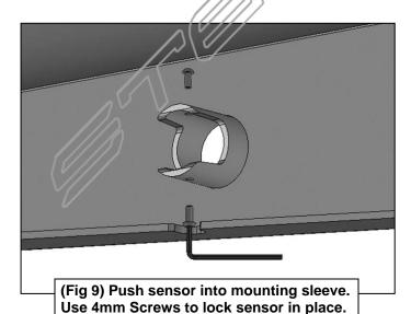
The 4mm Screws are only used to apply slight pressure to lock the sensors in place. Tighten both screws evenly until they touch the sensor body only. Do not overtighten screws or damage to sensors will result.
