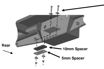
(Fig 7) Depending on model/year, the factory bumper may be attached to top of tow hitch, (see Figure 2). Attach mounting tab on back of Heavy Duty Bumper to top of hitch. Insert Spacer Plates (thin and/or thick) between tab and top of hitch to support the Bumper if necessary
