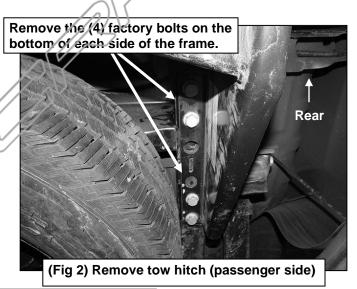
**WARNING!** Do not remove bumper bolts unless the bumper is properly supported on blocks or stands or the bumper may fall.
