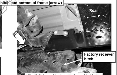
(Fig 8) Driver side installation with hitch
