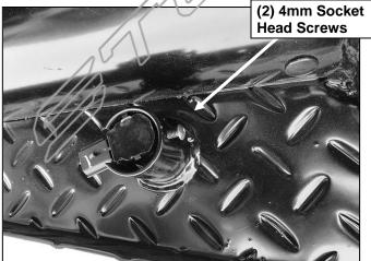
(Fig 11) Remove plugs from holes in bumper. Insert sensor (if equipped) into socket on back of bumper.
