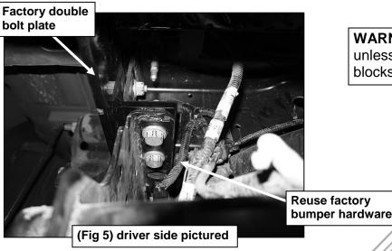
**WARNING!** Do not crawl under bumper unless the bumper is properly supported on blocks or stands or the bumper may fall.
