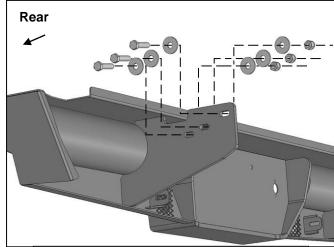
(Fig 6) Attach Bumper to outside of frame
