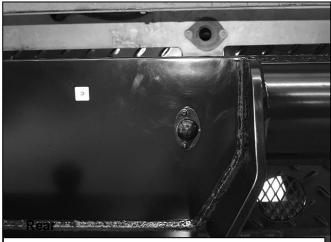
(Fig 5) Attach factory license plate lights to Bumper. Insert (2) Plastic Plugs for license plate
