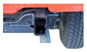
Put C type connecting plate into the passenger side
