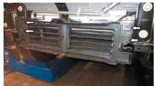
9. Unplug and remove the lower louvered air duct panel.
