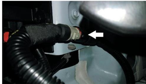
7. Lay the bumper down then remove the sensor and fog light wiring harness and block heater plug (if present) from the bumper. You will have to remove the (2) large black bumper support plates to remove sensors.
