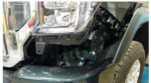
2. Remove the factory grille. Open the hood and remove the hood release latch by removing two T15 screws. Remove the ten plastic clips holding the plastic shield located above the grille.
