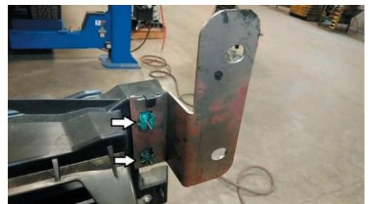
11. Remove the two black bumper mounting plate by removing the (4) 15mm bolts. The bolts will be used to install the Ranch Hand Frontend.
