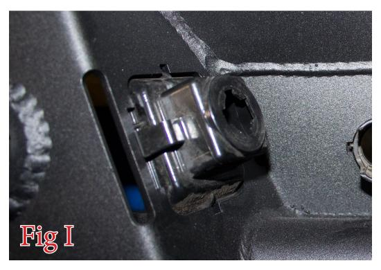
12. Install the parking sensor mounting rings onto your bumper by pressing them into their precut holes until they click into place. Make sure to install them in the same position/orientation as they came off your OEM bumper. If the rings do not click into place, you may have to trim the tabs on the sides of the mounting rings. (Fig J)
