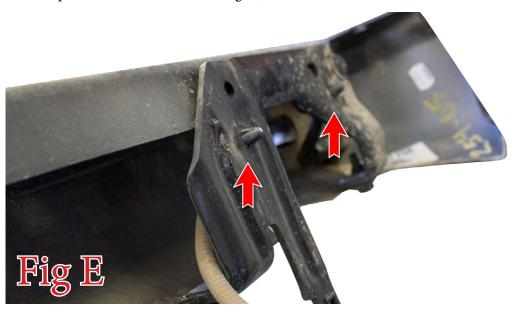
8. Grind the 5 welds to remove the license plate structure from the rear frame. Make sure to paint over any bare metal when you're done grinding. (Fig F)
