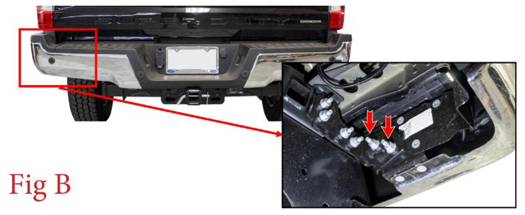
3. Remove the OEM Bumper Mounting Brackets. Use a 21mm Socket to remove the four mounting bolts (per side). Then, remove the brackets. (Fig C)
