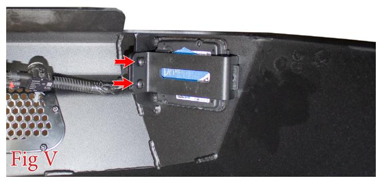
24. Install your Trailer Plug by pressing it into its precut hole until it clicks into place. If it does not click into place, you may have to spread the metal tabs on the back side of the trailer plug until they lock it into place. (Fig W)
