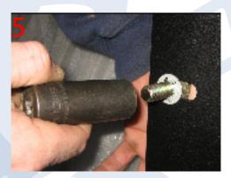
• Install the winch to the bumper using the supplied Allen Bolts and Washers. Note - Install the Flairlead bolts before you mount the winch.
