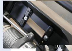
**Note** - Install the Flairlead bolts before you mount the winch.
