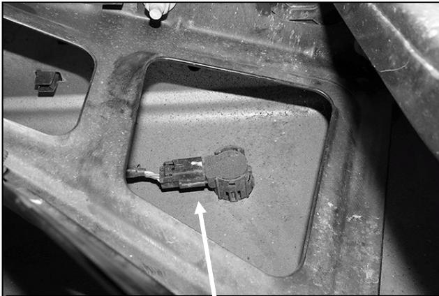
**(Fig 8) Unplug the sensor first then remove the sensor from the mount. Disassemble bumper to remove all sensors and harness as equipped**
