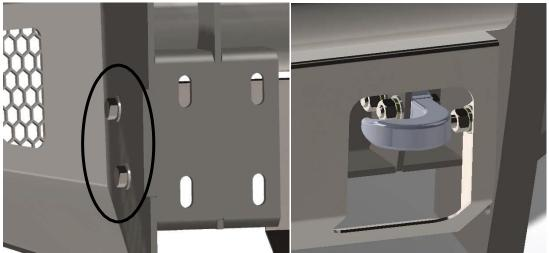
Figure 10a (bolt location for lower guard)
