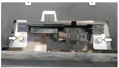
8. Before installing the Sport bumper, mount the sensor and factory bracket to the sensor bracket provided. Then mount the bracket to the tabs, using factory bolts, that was located behind the license plate.
