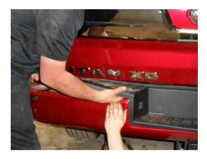
E. With the help of at least one more person, remove tailgate by removing the limit straps and camera harness from the bed. Then pull up on the driver's side of the tailgate with the tailgate approximately halfway open. Then slide the passenger side off the pivot point. This is at least a two
