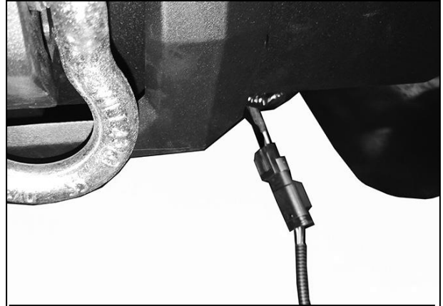
(Fig 15) Plug the long License Plate Light Harness into the factory wiring harness on the Bumper for the license plate light
