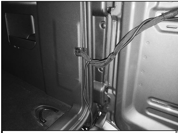
(Fig 16) Run the License Plate Harness over the door seal and up to the factory harness.
