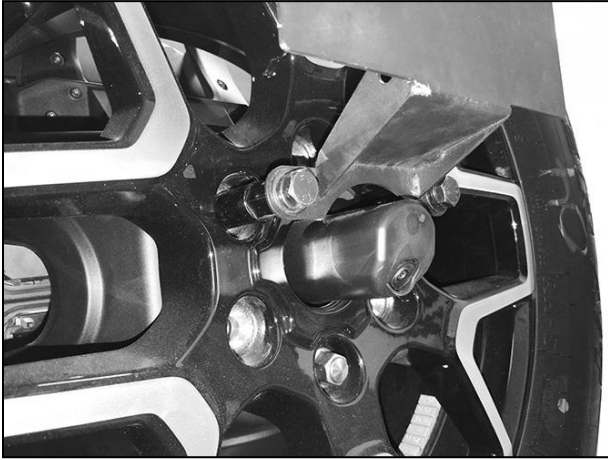
(Fig 19) Relocation Bracket installed
