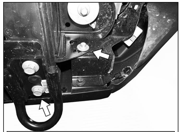
(Fig 2) Remove hex bolts attaching driver/left side bumper brackets to bottom of frame and side of body mount (arrows)
