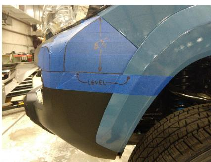
Figure 21 21. Using a silver sharpie, mark the bumper cover above the fog light pocket. (Figure 22)
