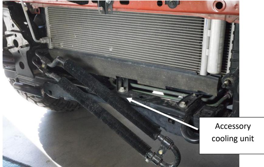
8. Remove the 8MM bolts that attaches the cooling unit to the frame.
