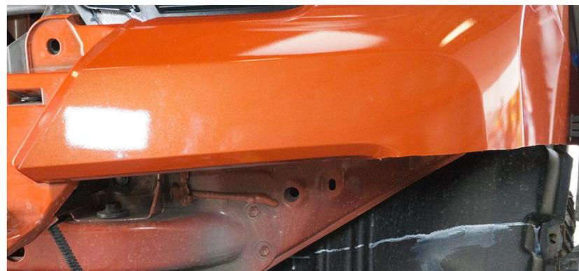
2. Make sure the line from the fog light pocket lines up at the fender below where the clip is on the fender flare. The lowest clip will be discarded with the bumper. The easiest method to mark the bumper is by using masking tape. The bottom edge of the tape is the cut line. Be careful when removing the tape so that the paint does not get damaged. Use a fine hacksaw blade or a utility knife to cut the polyurethane material.
