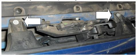
2 Remove all fasteners from wheel well top of bumper fascia, and from bottom of bumper fascia. If equipped with driving lights disconnect wiring harness at this time.
